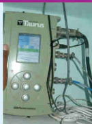
Seismograph for measurement of earthquake
